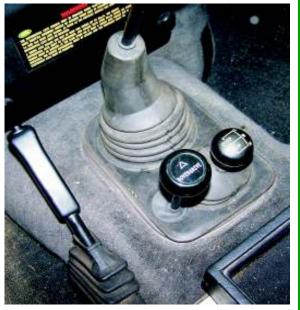
The distinctive third lever on the centre console of a Defender identifies it as a vehicle equipped with a ROAMERDRIVE overdrive.
